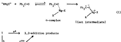
[Ph<sub>2</sub>Ċ-OMgX + R.] \_\_\_\_\_\_\_ d\*\* 1,6-Addition products escape from \_\_\_\_\_\_\_\_ pinacol + RH
